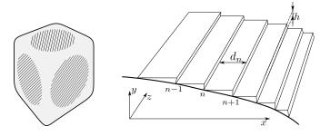
Equilibrium surface profile y(x) of a certain crystal and the corresponding microscopic staircase are shown schematically in the figure, where n denotes the step number, counting from x = 0. The profile shape at x > 0 can be approximated as  $y(x) = -(x/\lambda)^{3/2}h$ , where  $\lambda = 45 \,\mu\text{m}$  and  $h = 0.3 \,\text{nm}$ .
